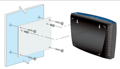
Figure 29. Wall Mounting the NetVanta 3200
